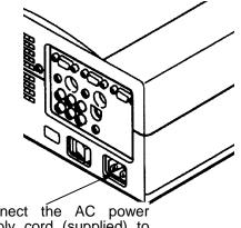
Connect the AC power supply cord (supplied) to the projector.
