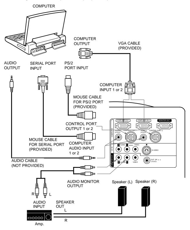
**NOTE**: The hook up should be done as per the above illustration. After hook up, turn on the projector, computer, in that order.
