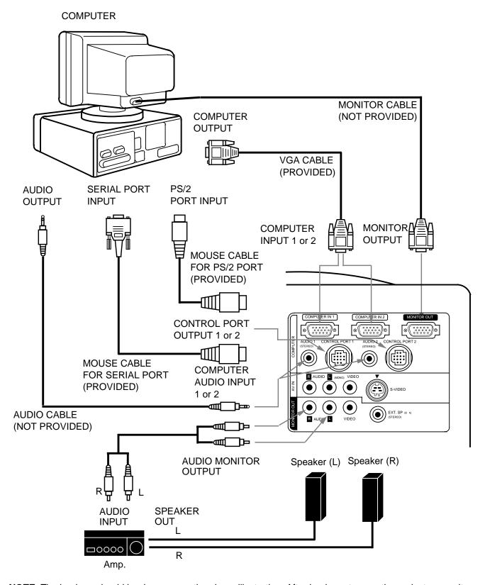
**NOTE**: The hook up should be done as per the above illustration. After hook up, turn on the projector, monitor, computer, in that order.
