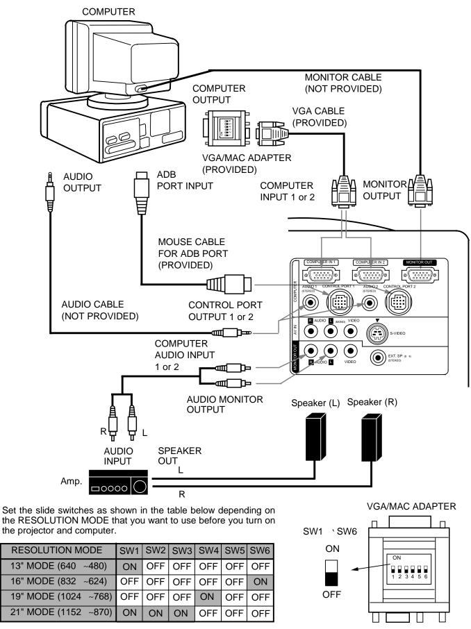
**NOTE**: The hook up should be done as per the above illustration. After hook up, turn on the projector, monitor, computer, in that order.
