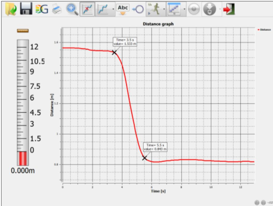
3. The first marker shows that when we started our recording we were 1.5 m away from the classroom wall; Then we moved towards the wall reaching a distance of 0.8 m - as we see on the 2<sup>nd</sup> marker.
